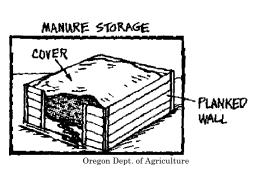
should have two to three walls to hold leached materials and to ease manure handling. Storage facilities should be located more than 100 feet from wetlands, streams, or ditches and above floodplains.
